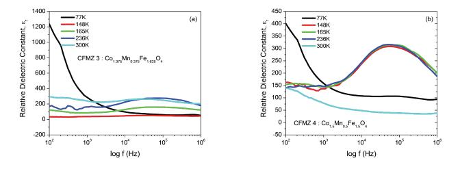
Figure-1: Relative dielectric constant of Co<sub>1+ x</sub>Mn<sub>x</sub>Fe<sub>2- x</sub>O<sub>4</sub>for (a) x=0.375 (b) x=0.5
